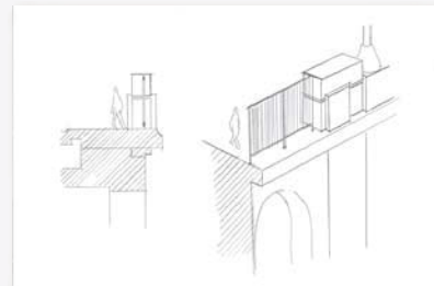
Option 10 - Replace railing & raise pilasters
