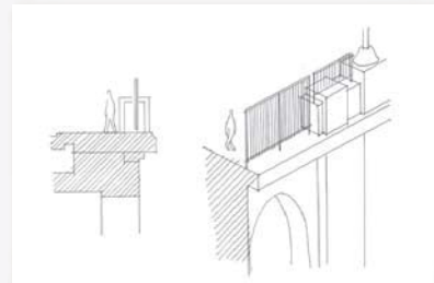
Option 7 - Replace with metal railing
